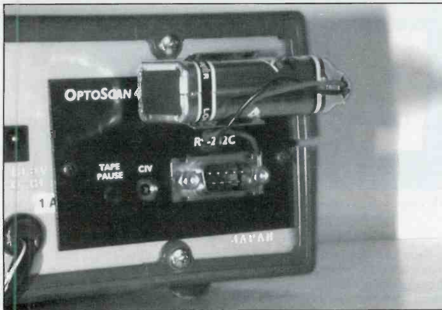
Rather than the recommended Velcro inside the radio, I chose to mount the battery on a clip outside the radio for convenience.
